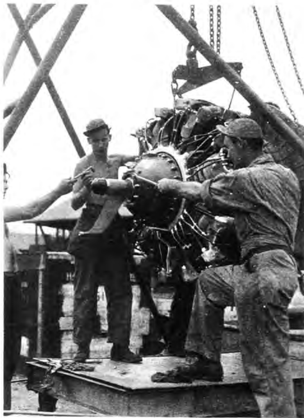
Above: Hoisting the new engine up before installing it.
